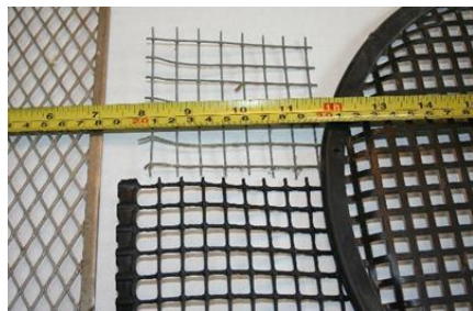
Figure 1. Different options for coarse mesh with openings of size between 8 and 12 mm to pass coarse aggregates before drying the soil fully.
