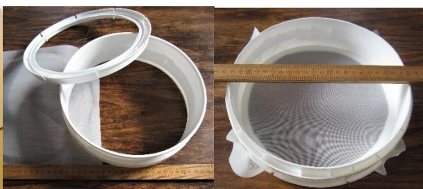
Figure 3. 0.25 mm or 250-micron sieve for the second sieving step in water, made from the top and lid of a plastic bucket, diameter between 20 and 25 cm.
