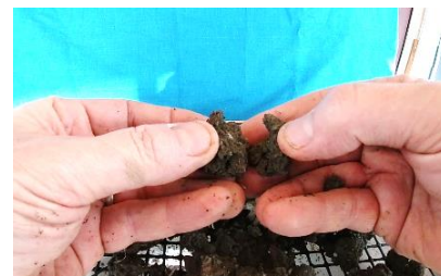
Figure 4. Breaking large aggregates along planes of natural weakness in the soil, to make aggregates that pass the large mesh (8-12 mm)
